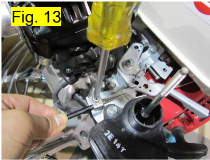
Step 10: Secure the wire to the cable clamp while pushing with slight pressure forward. (Fig. 13)
