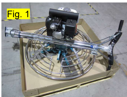
Step 1: Trowel shown with handle separate. (Fig. 1)
