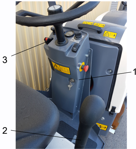
Fig. Instrument panel 1. Starter switch 2. Engine speed control 3. Parking brake
