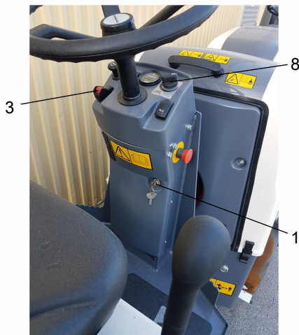
Figure. Instrument panel 1. Ignition key 3. Parking brake 8. Switch, sprinkler
