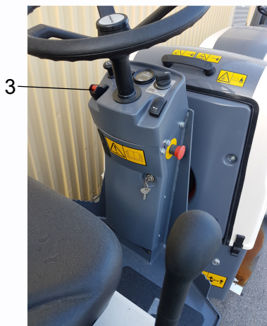
Fig. Control panel 3. Parking brake 12. Parking brake warning lamp
