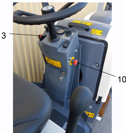
Fig. Controls 3. Parking brake 10. Emergency stop
