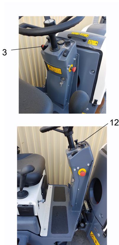
Figure. Instrument panel 3. Parking brake 12. Brake warning lamp
