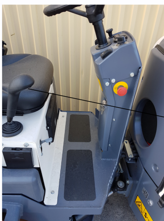
Fig. Forward/Reverse lever 4. Switch, vibration On/Off
