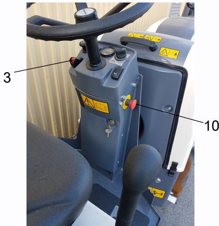
Figure. Control panel 3. Parking brake 10. Emergency stop
