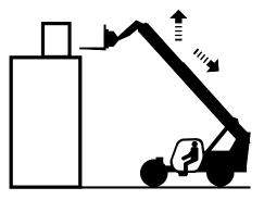
8 When the forks are clear of the load and the structure, the boom can be lowered and retracted.
