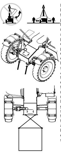
Do not permit the load to swing freely. Always properly tether loads to restrict movement. In addition to ground personnel, the two chassis tie-down points in the front of the machine can be used to help externally stabilize the load. Always cross the tethers to opposite sides of the load to minimize load movement. Driving across grades, sudden starts, stops, and turns can cause the load to swing and create a hazard if not externally stabilized.
