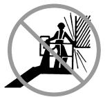
Be aware of crushing hazards when grasping the platform guard rail. During movement of the platform, occupants must keep all body parts inside the platform railing.
