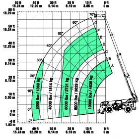
\* Load Capacities are at 24\*/60cm load center from forward edge of Adapter \* Weight and center of gravity of attachment should be considered part of rated load
