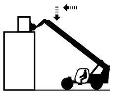
7 Gradually move the controller to raise and retract the boom. This will bring the forks out of the load.
