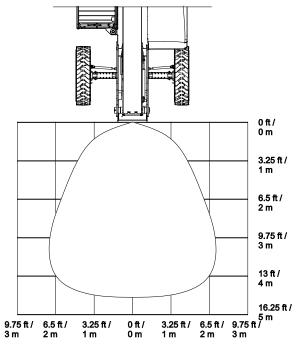
Approximate detection range. Minimum rear proximity sensor detection height is 2 ft / 0.6 m.
