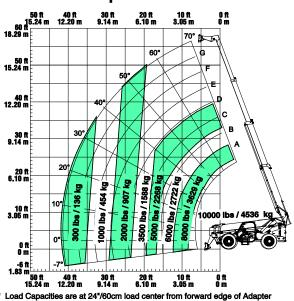
Load Capacities are at 24"/60cm load center from forward edge of Adapter
